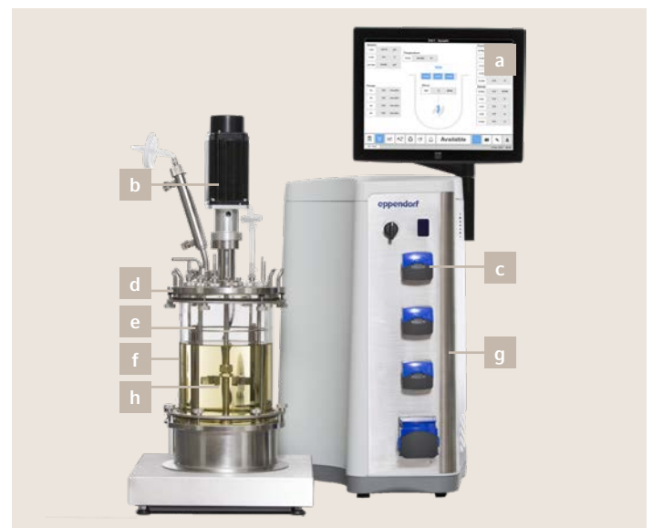
Figure 11: Composition of a bioreactor. Components of a stirred tank-bioreactor (left) and a connected control station (right).
